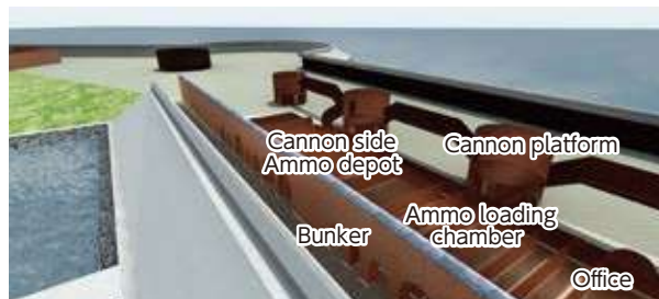
Chart 10 : Underground construction image of the bunker (CG)
